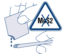
Oil hub and shaft lightly, if necessary ( do not use oil containing MoS2 ).
